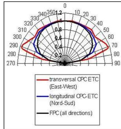
Illustration 3: Collector efficiency curves for plasma coated CPC-ETC collectors and the dependence of the radiation incident angle on the fraction of used radiation for CPC-ETC and for flat collectors
