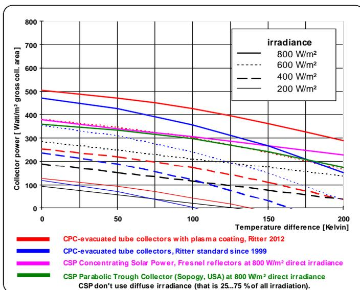
Illustration 5 – Efficiency curves of CPC-ETC, Fresnel reflector and parabolic trough collectors
