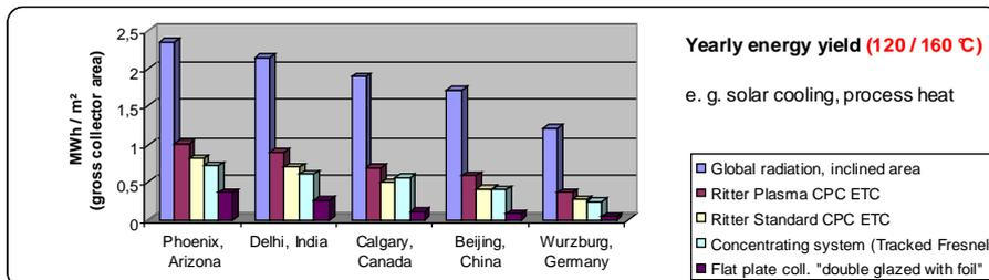
Illustration 7 – One year T\*SOL simulations for different temperatures, sites and collector systems
